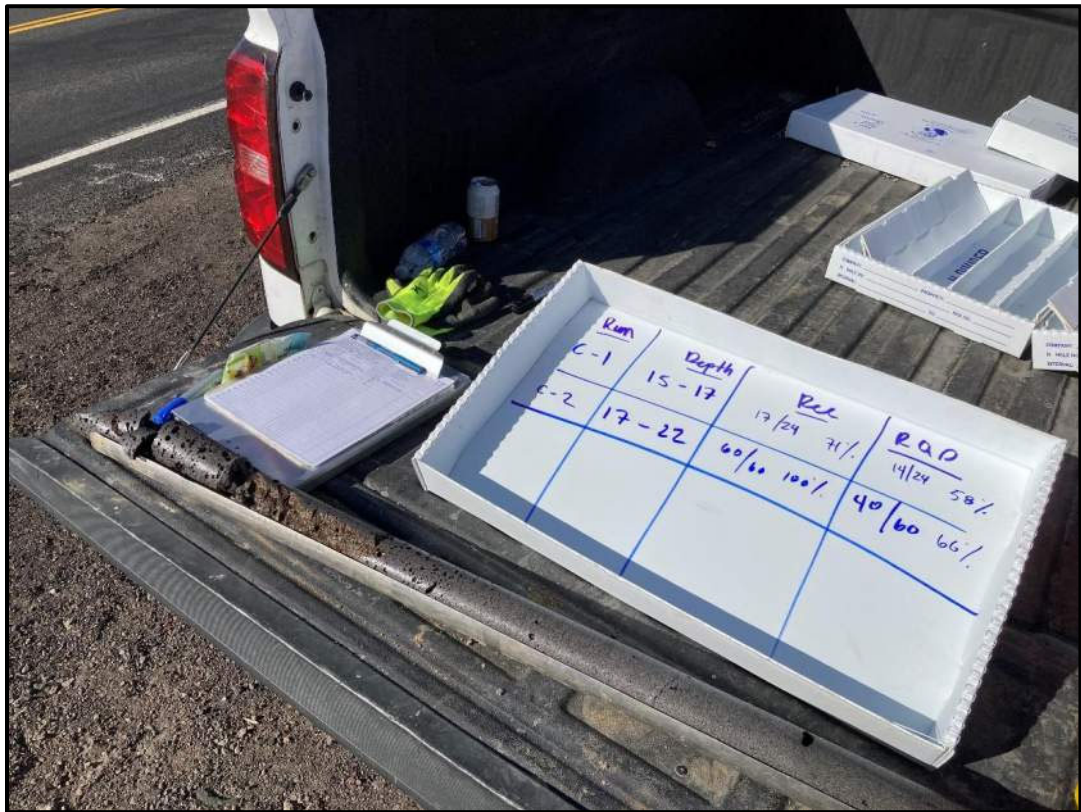
B-02 core run C-2 from 17 to 22-feet bgs. Note transition to massive rock with very few vesicles.
