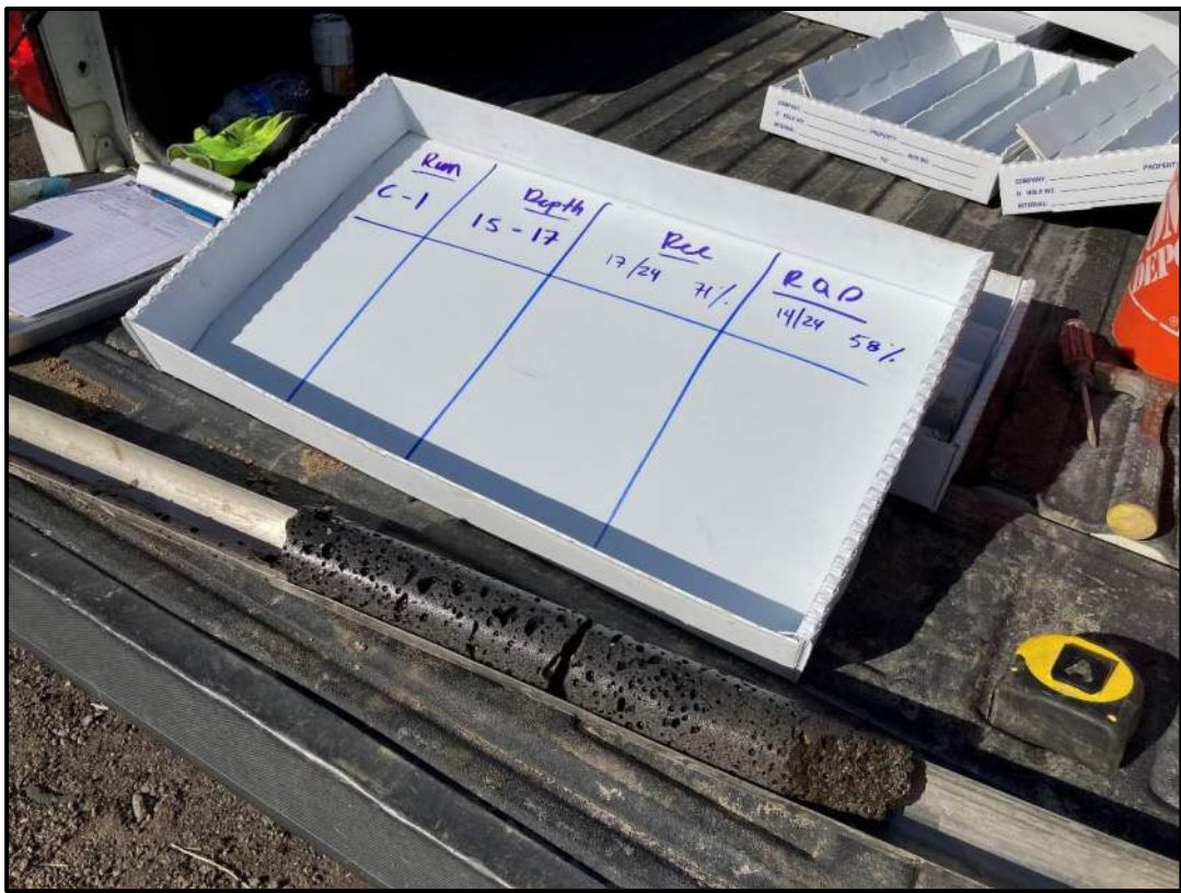
B-02 core run C-1 from 15 to 17-feet bgs. Note abundant and large vesicles.
