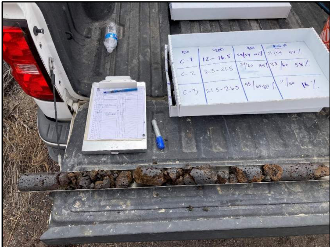
B-01 core run C-3 from 21.5 to 26.5-feet bgs. Note very poor rock quality.
